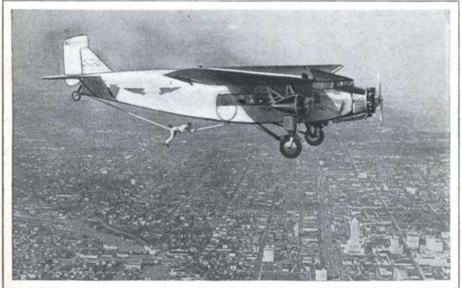
With the aid of this safety device, experienced mechanics can make repairs on planes in flight. Ordinarily landings are necessary in the event of trouble with tail surfaces but are now eliminated.
